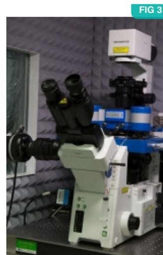
FIG 3 FM microscope JPK NanoWizard 4XP installed on a Leica DMI8 optical microscope with a fluorescence module at CF Nanobio (CEITEC).
