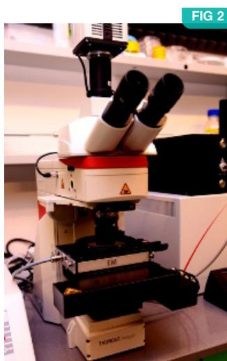
FIG 2 New cryo-fluorescence microscope for imaging of fluorescently labeled samples at cryo-conditions installed in 2021 at CEITEC.
