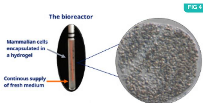
**FIG 4** The assembled in-cell NMR bioreactor containing encapsulated mammalian cells and the inlet tube for fresh medium supply (left) and a slice of the hydrogel thread showing the encapsulated cells (right).
