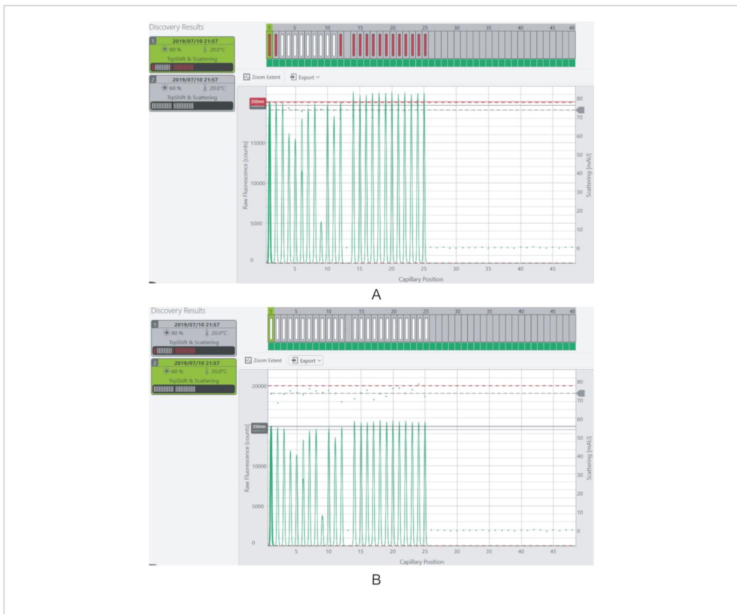
Figure 4: Adjusting the excitation power and fluorescence signal. (A) At 80% excitation power, the fluorescence signal for most of the samples is beyond the saturation limit. (B) The fluorescence signal is reduced to measurable levels by decreasing the excitation power to 60%. Please click here to view a larger version of this figure.
