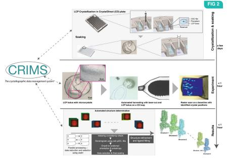
The joint EMBL Grenoble - ESRF structural Biology group (JSBG) is currently involved in the installation of a CrystalDirect harvester on the ID30A-1/MASSIF-1 beam line to enable plate-to-beam data collection modes, and in the upgrade of ID29 to a dedicated high brilliance serial synchrotron crystallography beam line for challenging dynamic structural biology projects. User access to CrystalDirect at MASSIF1 and to the ID29 beam line is expected to start in summer 2022.
