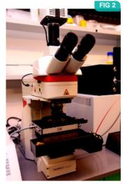
**FIG 3** FM microscope JPK NanoWizard 4XP installed on a Leica DMi8 optical microscope with a fluorescence module at CF Nanobio (CEITEC).
