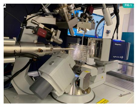
FIG 1. (A) Rigaku Liquid Metal Jet (LMJ) Synergy System with an Excillum LMJ source and Rigaku HyPix Arc 150°-pixel detector operating at the Weizmann Institute Instruct-ERIC Center. (B) Ligand binding to Quinone Reductase 2 (hQR2) (paper in preparation).
